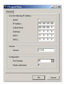
This page enables to define all IP parameters of the Power Switch 1-port device and displays the version of the Firmware. The HTTP protocol is enabled and the Finder program is authorized at factory settings.
