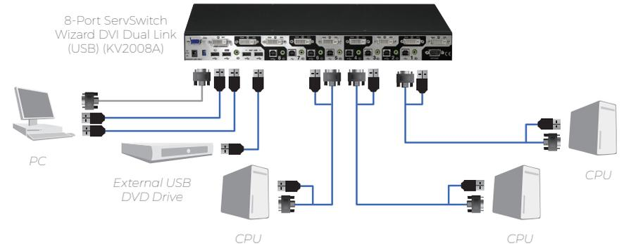
on the switch's console port plus two USB 2.0 transparent ports for any USB 2.0 peripherals.
