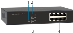
Figure 4-1. LEDs on front panel of switch.
