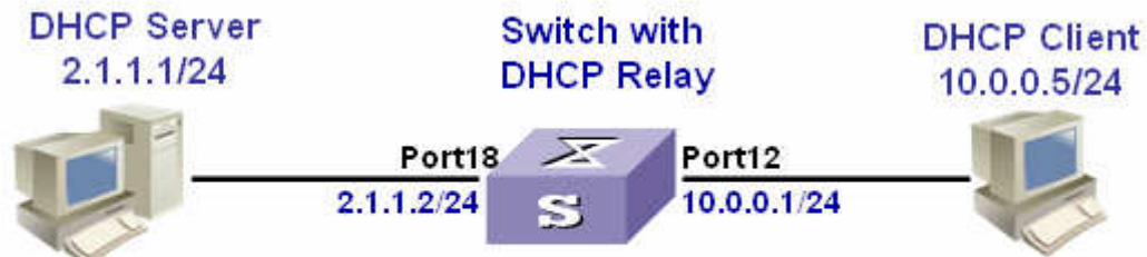
An example of DHCP Relay
