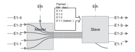
Figure. 3.14 Automatic configuration, 4x E1 and Ethernet are transmitted over one SHDSL link
