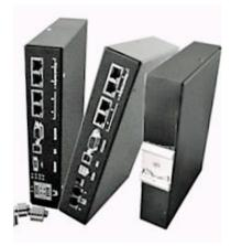
All LED to recognize the behavior and see the status of the DT/DR device are integrated in the connectors. On the black ABS enclosure there are also some additional LED's on the front panel.
