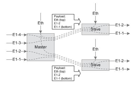
Figure 3.15 Automatic configuration Star-topology
