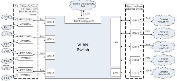
Figure 3.20 Internal Switch (ETH5 is not available for DT/DR devices)
