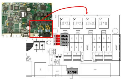
Figure 3.10 Default Jumper position and LP/DP switch position
