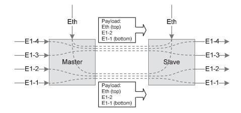
Figure. 3.16 Automatic configuration 2x E1 and Ethernet are transmitted over two SHDSL link.
