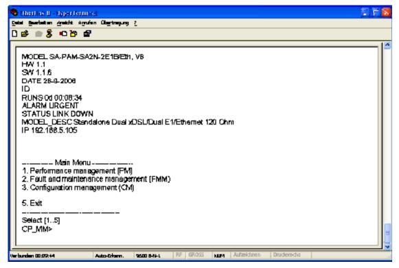
11. Go to the "Fault and maintenance management" menu, means to enter number 2. Enter the <SOFTUPDATE> command. After typing SOFTUPDATE, the device tries to establish connection over the X-modem protocol within 60 seconds.
