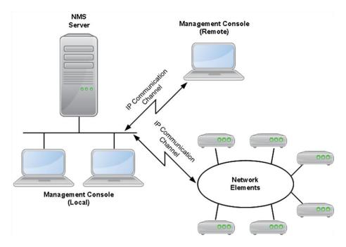
Figure 0.132 The structure of SNMP-based NMS.
