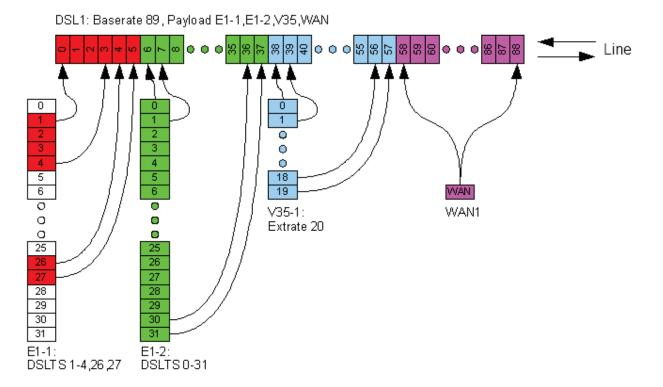
Figure 3.24 Example of distribution of time slots in an SHDSL frame at a line rate of 89x64 kbit/s in the mode when both E1 interfaces 1280 kbps of V.35 and both internal WAN1 and WAN2 ports are used for the termination device.
