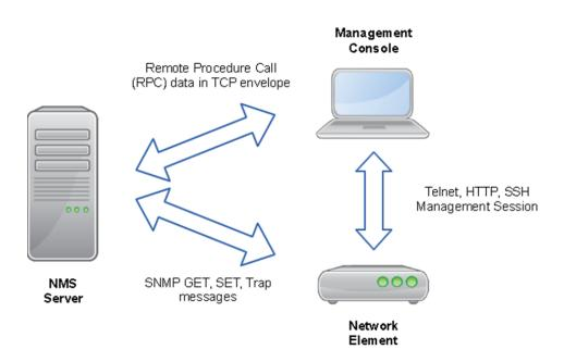
Figure 0.233 Message exchange in SNMP-based networks.
