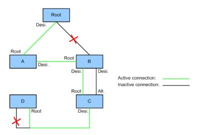
Figure 3.23 Change of Port role upon network failure.
