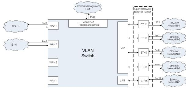
Figure 3.21 Internal Switch for single-channel devices (SA-DT-ETH\_IV-SRL-2E1B/4Eth-RP,V90)
